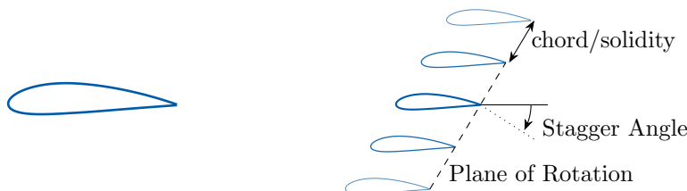
Figure 2: An isolated airfoil (left) differs from a linear cascade of airfoils (right) in that the airfoils in the cascade are influenced by the airfoils coming before and after (with decreasing influence out to infinity). The spacing between airfoils is determined by the blade section local solidity, and the skew of the cascade is determined by the stagger angle of the blade section.
