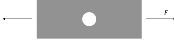
Figure 2.30: A plate with a hole experiences stress concentrations near the hole.
