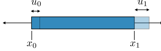
Figure 1.7: A more general representation of one-dimensional strain where both ends of the bar displace.
