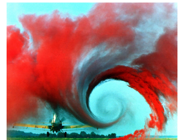
Fig. 4.6 Picture of aircraft flying through colored smoke to visualize the wake vortex. Picture from NASA, public domain.
