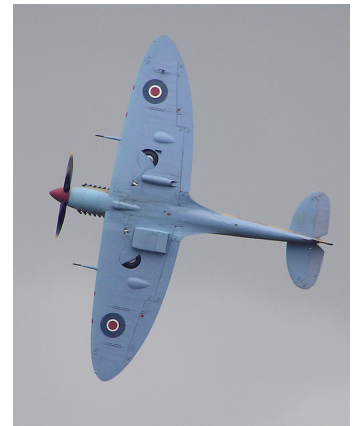
Fig. 4.21 The Supermarine Spitfire is a well-known example of an aircraft with an elliptic wing. Image from Adrian Pingstone , Wikimedia, public domain.
