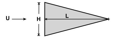
Compute the drag coefficient assuming a Reynolds number based on length of the plate of  $Re_L=5e5$ . The reference area for the drag coefficient should be the triangular planform area. Return your answer in "counts" of drag. One count is 1/10,000 or in other words  $C_D=0.00123$  would be 12.3 counts of drag.
